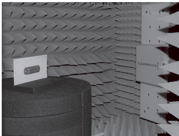
Figure 6: The RFID measurement cabinet inside, turntable with a blue RFID-transponder on a white plastic substrate to the left; linear polarized reader-antenna on the right; surrounding absorbers
