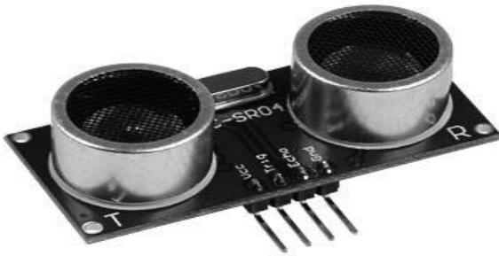
Figure 3 Example of an ultrasonic sensor
