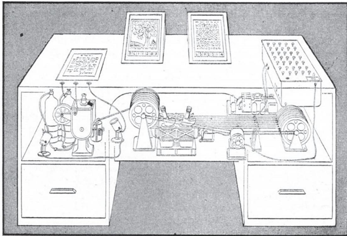
**MEMEX** in the form of a desk would instantly bring files and material on any subject to the operator's fingertips. Slanting translucent viewing screens magnify supermicrofilm filed by code numbers. At left is a mechanism which automatically photographs longhand notes, pictures and letters, then files them in the desk for future reference.
